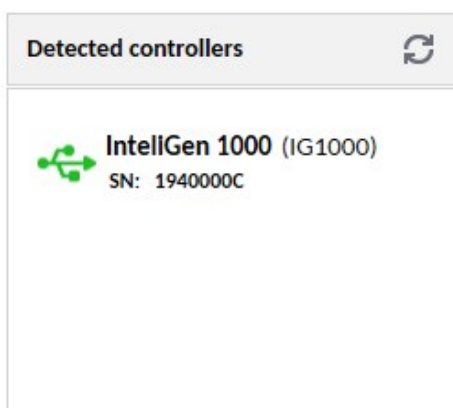
Image 5.2 Second screen of IntelliConfig - Select your controller from list of Detected controllers.
